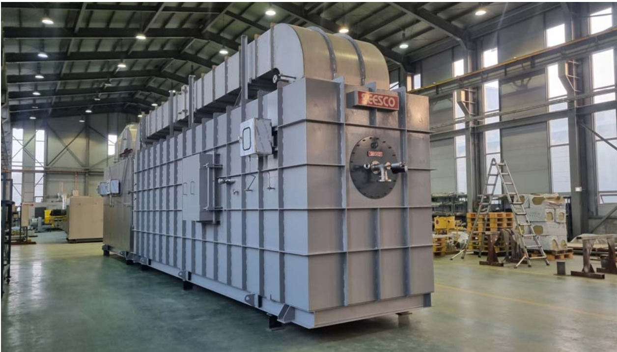
SDTO Thermal Oxidizer with Heat Exchanger for Petro-Chemical process
