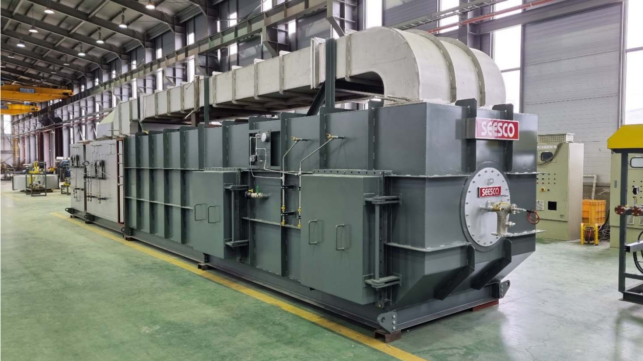
SDTO Thermal Oxidizer with Heat Exchanger for Automobile paint dry oven 2 nd Heat Exchanger for a zone heating of dry oven
