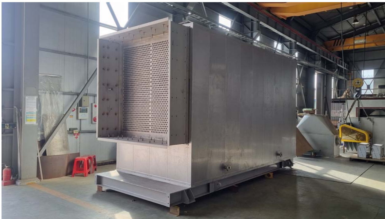
Tubular Type Heat Exchanger for SDTO Thermal Oxidizer
