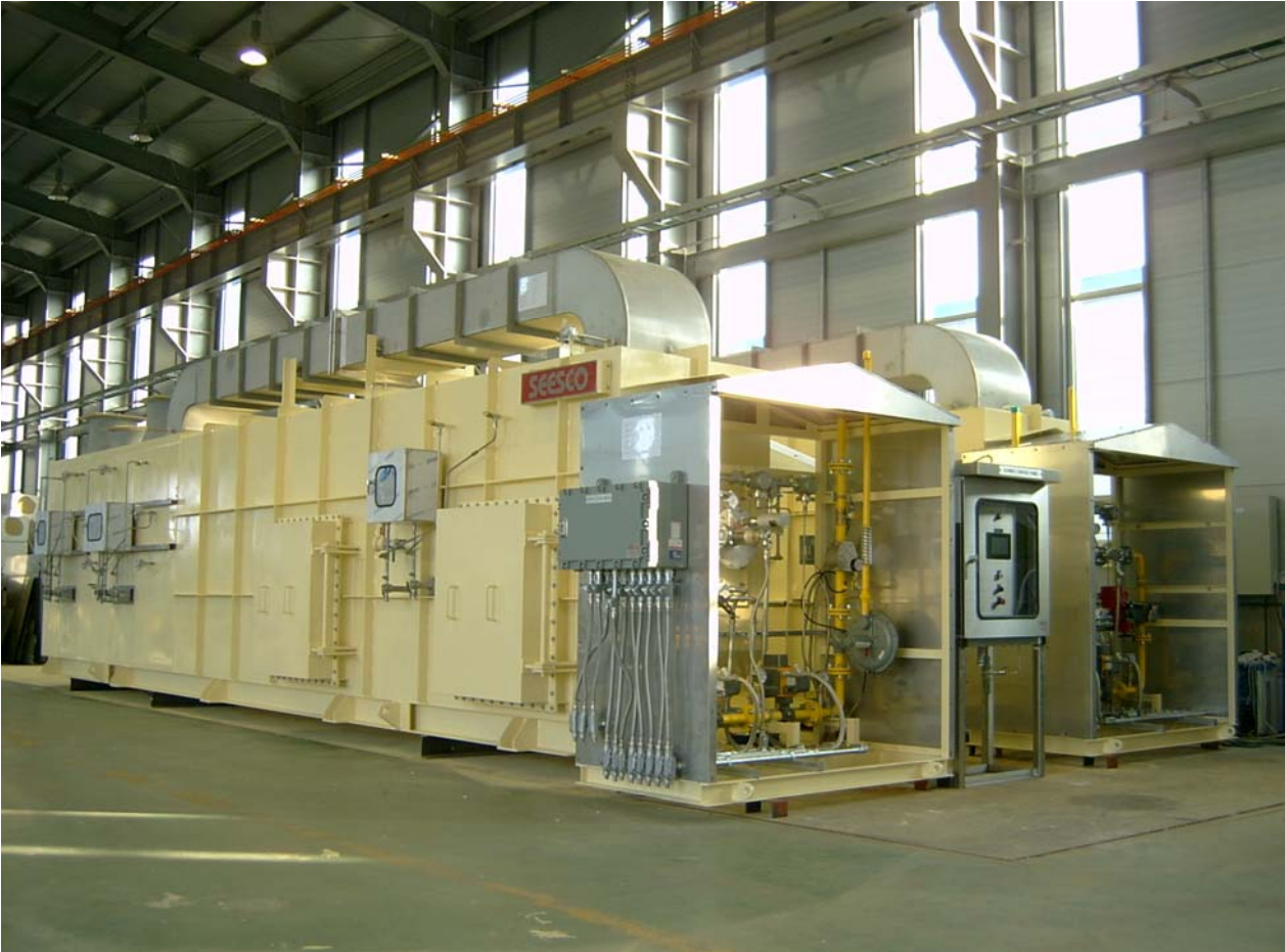
SDTO Thermal Oxidizer with Heat Exchanger for LCD process
